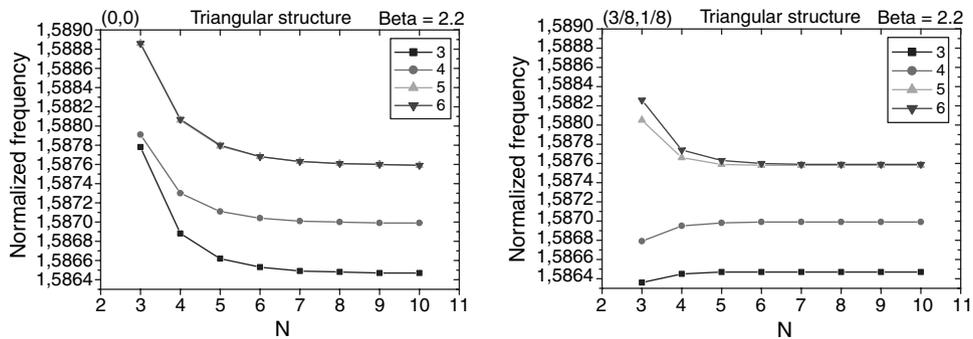
**Fig. 2.** Convergence with supercell size of the guided-mode eigenfrequency for an index-guiding PCF with the air holes arranged in a triangular structure with  $d/\Lambda = 0.6$ . The graph shows the normalized frequency as a function of  $N$  with  $\beta = 1$ . The calculations for the CR  $k$ -point  $(3/8, 1/8)$  (right) all show better convergence compared to  $\Gamma$ -point calculations (left).
