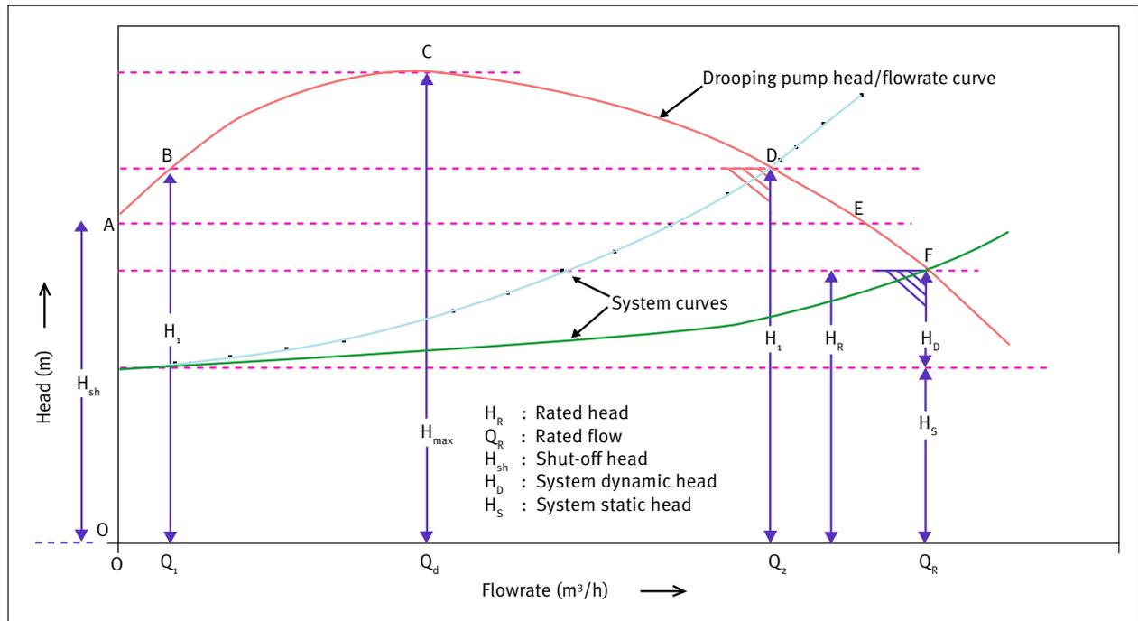
Figure 2. Condition to determine acceptance of a pump with a drooping head/flow rate curve.
