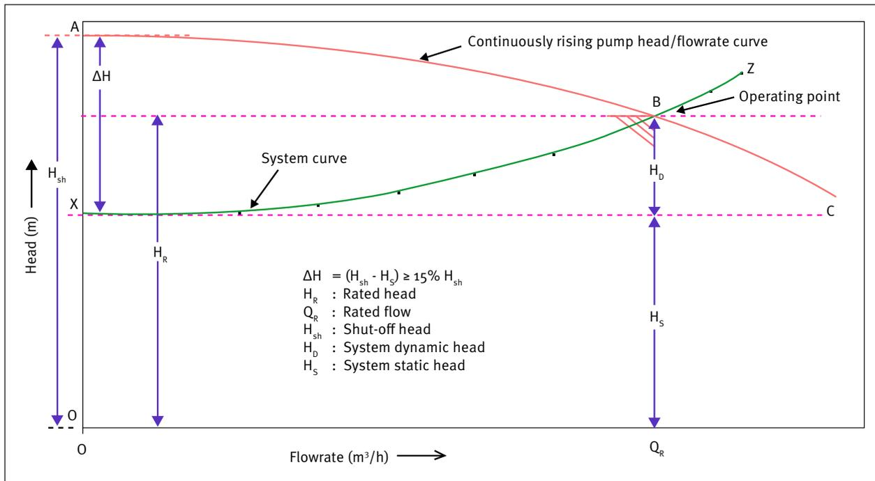
Figure 1. Condition to determine the permissible pump head rise.
