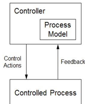
Fig. 2. Leveson’s control model of system safety.<sup>2</sup>
